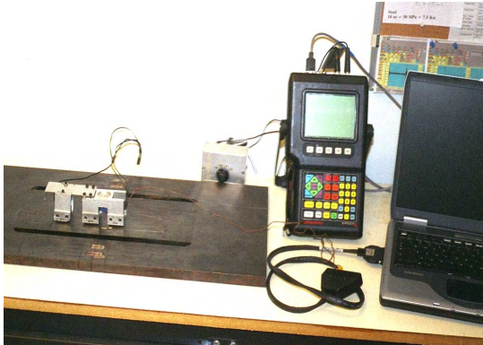
Figure 1 Test setup for L_{CR} ultrasonic stress measurement
