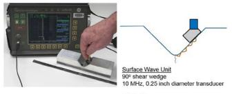
Calibration 80%FSH from 0.02 x 0.01 inch notch in a 7075-T7 reference plate
