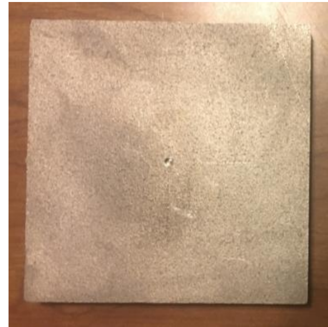
Hole Drilling Location on Substrate Back Surface
